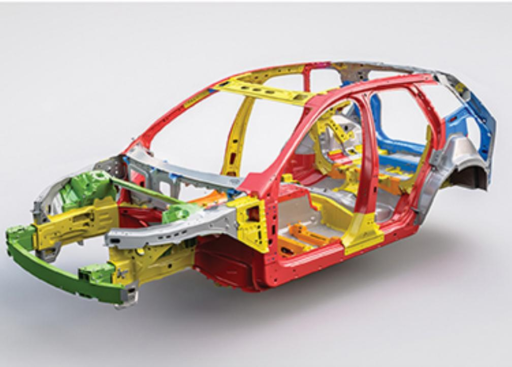
The body of the XC60 provides you and your passengers with maximum protection in all types of accidents and uses a high percentage of ultra high-strength boron steel to create a protective cage around you and your passengers.
